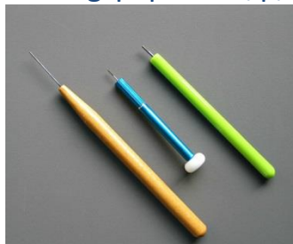
Quilling Tools: left to right: needle tool, ultra-fine slotted tool, slotted tool
